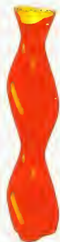
Figure 2. Capillary instability of a nanowire with an anisotropic surface energy with three-fold symmetry about the wire axis.
